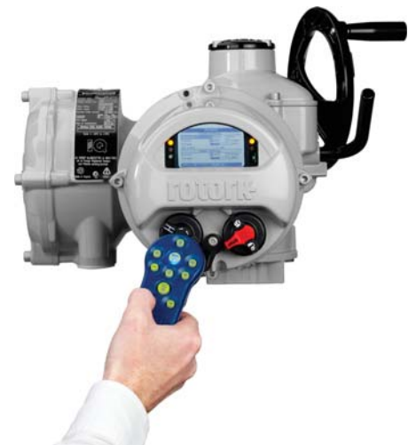
Fig 3: Rotork IQ3 intelligent electric valve actuator with non-intrusive bi-directional hand held setting tool for setting up, commissioning, monitoring, adjustment and downloading of data logger records for diagnostics and asset management. Rotork IQ, CVA and Skilmatic electric actuator designs share versions of this technology.
