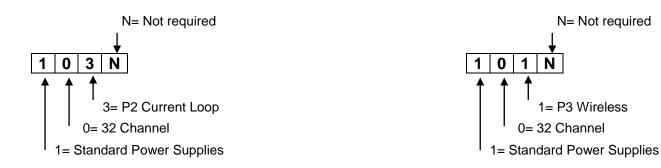
Backplane: If you specify 'Not required' (=N) for the backplane, no backplane will be supplied. Any other items will be supplied loose, i.e. as spares. If you specify '1' the backplane will be supplied with the standard power supply (87 to 265 Vac), if you specify 2 the backplane will be supplied with a DC power supply (18 to 36 VDC).
