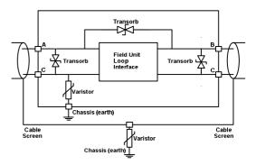
In addition, all the loop circuit components and field connections are optically isolated from the processor. This ensures that a failure of the field unit detector circuits is not transmitted to the circuits of the attached actuator, allowing it to continue functioning.
