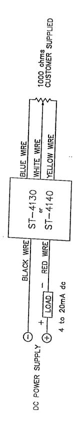
INPUT POWER: 12.0 (MIN) TO 36Vdc (MAX), 25mA.
