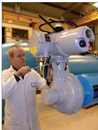
Blackhall engineer Tom Scanlon completes the mechanical installation of one of the Rotork IQM actuators (left). The size of the two valves is apparent in this workshop view (right).
