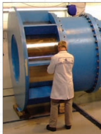
Blackhall engineer Tom Scanlon completes the mechanical installation of one of the Rotork IQM actuators (left). The size of the two valves is apparent in this workshop view (right).
