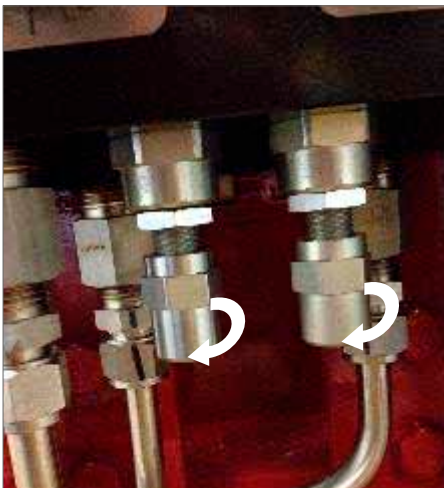
Fig 12.6 Flow regulator cap removal
