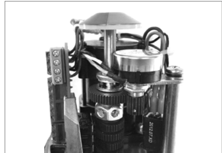
Mechanical ROM cover removed
