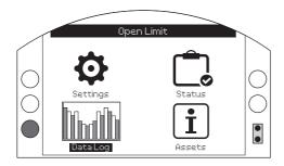
The data can be viewed locally on the dot matrix display from pressure and position graphs through to statistical operational data. All data held is secure and can be downloaded using the Rotork Bluetooth® Setting Tool *Pro* for viewing on a PC with Rotork Insight 2 software.
