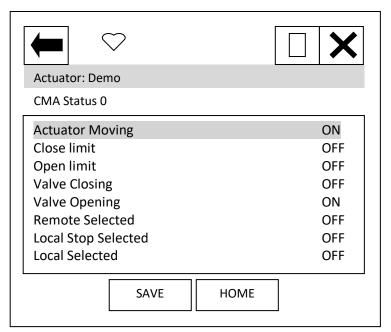
'Actuator Moving' indicates that the actuator is currently moving.
