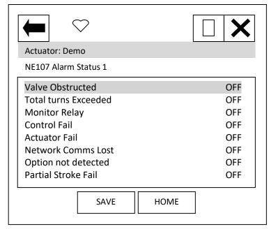
'Valve Obstructed' indicates that the actuator has tripped/stopped on torque due to an obstruction in the valve.
