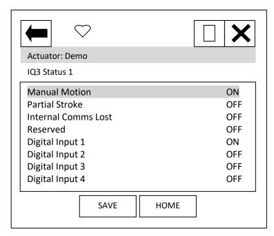
'Manual Motion' indicates that the actuator is currently moving under manual control.
