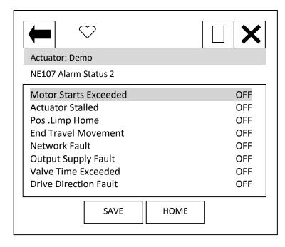
'Motor Starts Exceeded' indicates that the limit for the number for motor starts expected in the actuator life has been exceeded.
