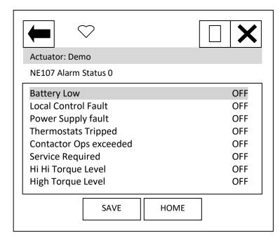
'Battery Low' indicates that the actuator battery used to maintain the display, is either flat or low.
