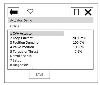
Item 1 'CVA Actuator' indicates the type of actuator. CVL for Linear CVA and CVQ for quarter turn.
