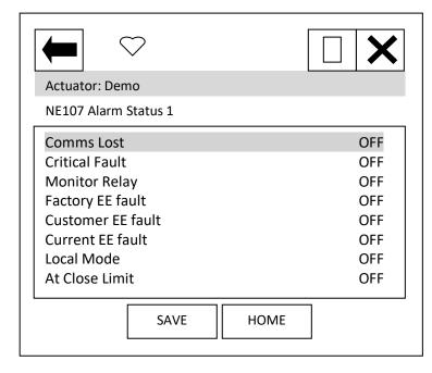
'Comms Lost' indicates that the network card is not able to communicate on the network – this is unlikely to be seen.
