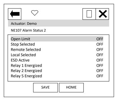
'Open Limit' indicates that the actuator is at the open limit.
