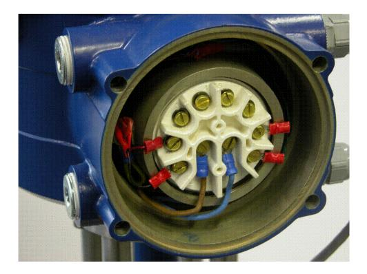
Network connections are made to the terminals of the actuator. Shown above is a typical arrangement for a CVA range actuator. HART is connected to terminals 1 and 2. Always check the actuator wiring diagram for correct terminal numbering and connection polarity.
