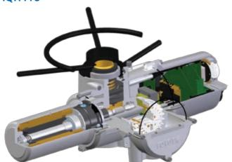
\*Note: It should be noted that a self-locking ability cannot be guaranteed for worm and wheel drives under all conditions including high loads and vibration, either under static and dynamic conditions. When handwheel operation is selected the gear train is disconnected and therefore any locking ability will be lost.
