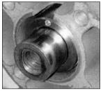
Fig. 4.9 Type A Drive Bush in Position 2
