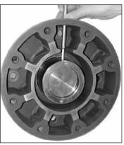
Fig. 4.12 Tightening Retainer Set Screw
