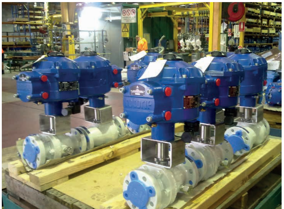
CVA actuators at the valvemakers factory awaiting shipment to site.
