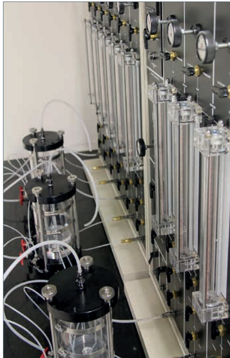
Panel mounted Fairchild Model 10 Regulators are used on the 'Measurement of index flux through saturated geo-synthetic clay liner specimens using a flexible wall permeameter' test rig at TRI Australasia.
