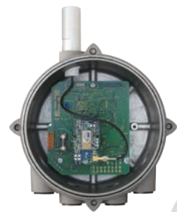
IQ Pro actuator showing Pakscan P3 wireless network card installed.
