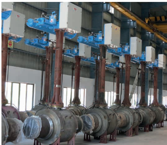
Rotork GP actuators mounted on 30 inch pipeline ball valves await shipment from the valvemaker's factory for buried service installations on the Kochi-Kootanad Bangalore-Mangalore Pipeline.
