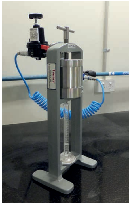
The Fairchild Model 10 Regulator is also used on the test instrument for 'Fluid loss of clay component of geo-synthetic clay liners'.
