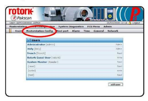
The following screen enables the PIN and level of protection to be set, shown circled in red. See above section for details of the levels of protection that can be set. Note that the current PIN will be shown, so to prevent access to this information, the web pages should either be disabled or the login password changed.
