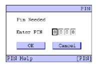
To enter a PIN, or accept the number, press ENTER and the first digit will flash. The value can be changed by using the left or right arrow keys. Once the number is correct, press ENTER once more. When all 4 digits of the PIN are entered correctly, select the OK button with the arrow keys and press ENTER.
