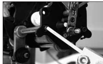
Fig. 10.2 AOP Front Plate Fixing Screws
