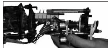
Fig. 10.4 AOP re-alignment and engagement
