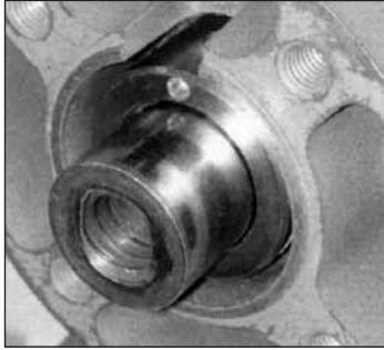
Fig. 5.7 Type A Drive Bush in Position 2
