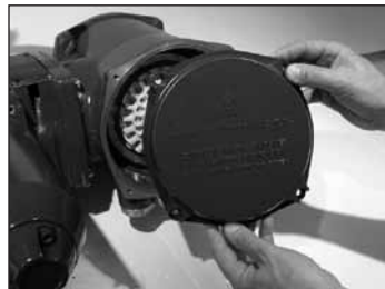
Fig. 7.1 Removing the terminal cover-Syncropak
