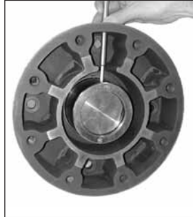
Fig. 5.9 Tightening Retainer Set Screw
