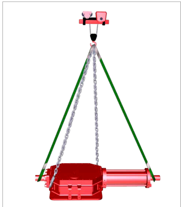
Fig 7.4 Lifting (double-acting actuator size 200 - 350)
