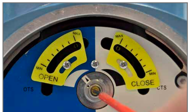
Torque cam clutch screw adjustment.
