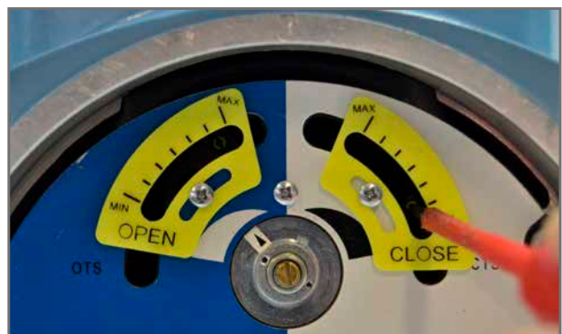
Close torque setting adjustment.
