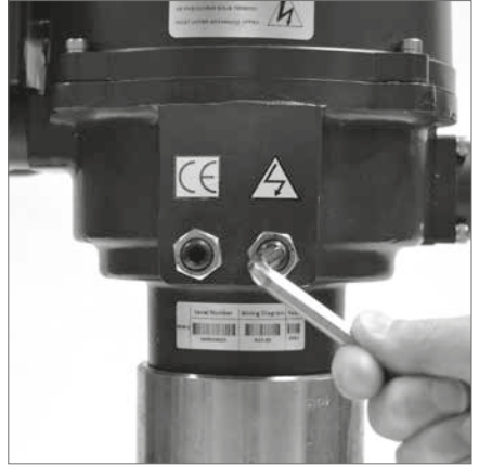
Setting clockwise to close stop bolt
