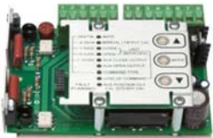
Positioner PCU DHC-100D without feed back signal incl. mounting
