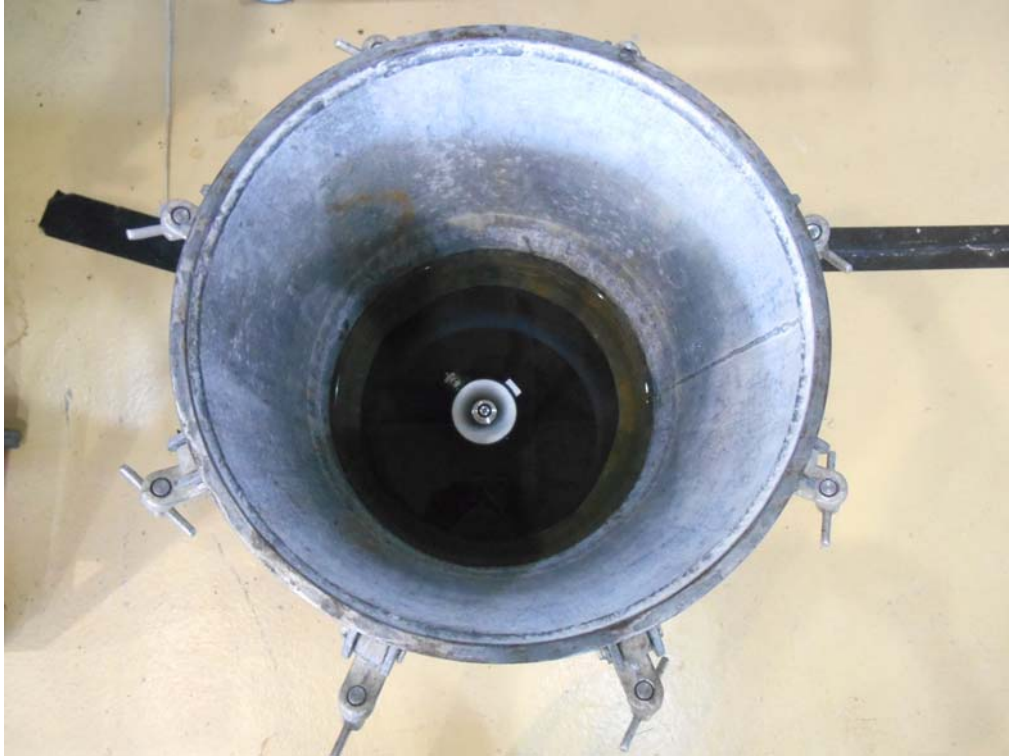
IPX8 INGRESS PROTECTION - PRESSURE CYLINDER – SPECIMEN CONFIGURATION
