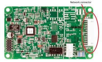
Fig. 3: The Profibus single channel NIC, showing the network connector
