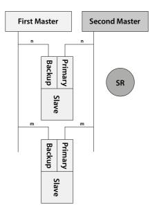
Fig. 9: Profibus DP System Redundancy Connection
