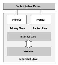
Fig. 7: Profibus DP Simple Dual Redundant Option Block Diagram
