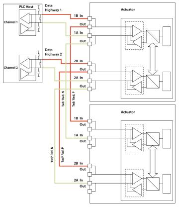
Fig. 13: Dual Highway SR Mode Connections
