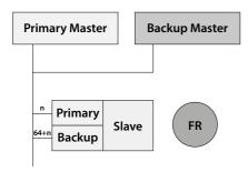
Fig. 8: Profibus DP Flying Redundancy Connection
