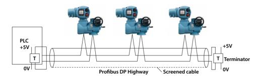
Fig. 5: Typical Profibus DP Data Highway
