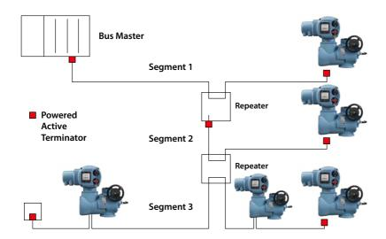
Fig. 6: Profibus Single Channel Data Highway Topology
