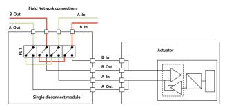
Fig. 15: Disconnect module showing unpowered operation disconnected from the actuator.
