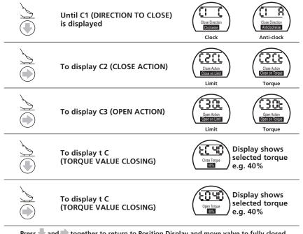
Press  $\P$  and  $\blacksquare$  together to return to Position Display and move valve to fully closed condition checking that closed symbol and lamp appear just as the limit of travel is reached.
