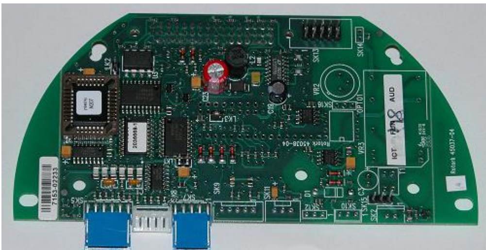
Fig 3: The FF01 Mk2 interface Card (Q and Skil/EH actuators)
