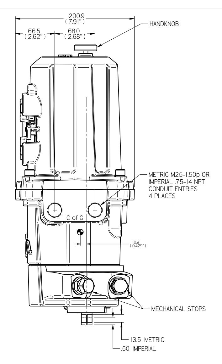
NOTES: 1) ALL DIMENSIONS ARE IN mm WITH CONVERSION FOR (INCHES). 2) CMA ACTUATORS CAN BE SELECTED WITH EITHER METRIC OR IMPERIAL SIZES FOR THE SHAFT AND CONDUIT ENTRY. THESE ARE NOT SIMPLE CONVERSIONS BUT DIFFERENT DIMENSIONS.
