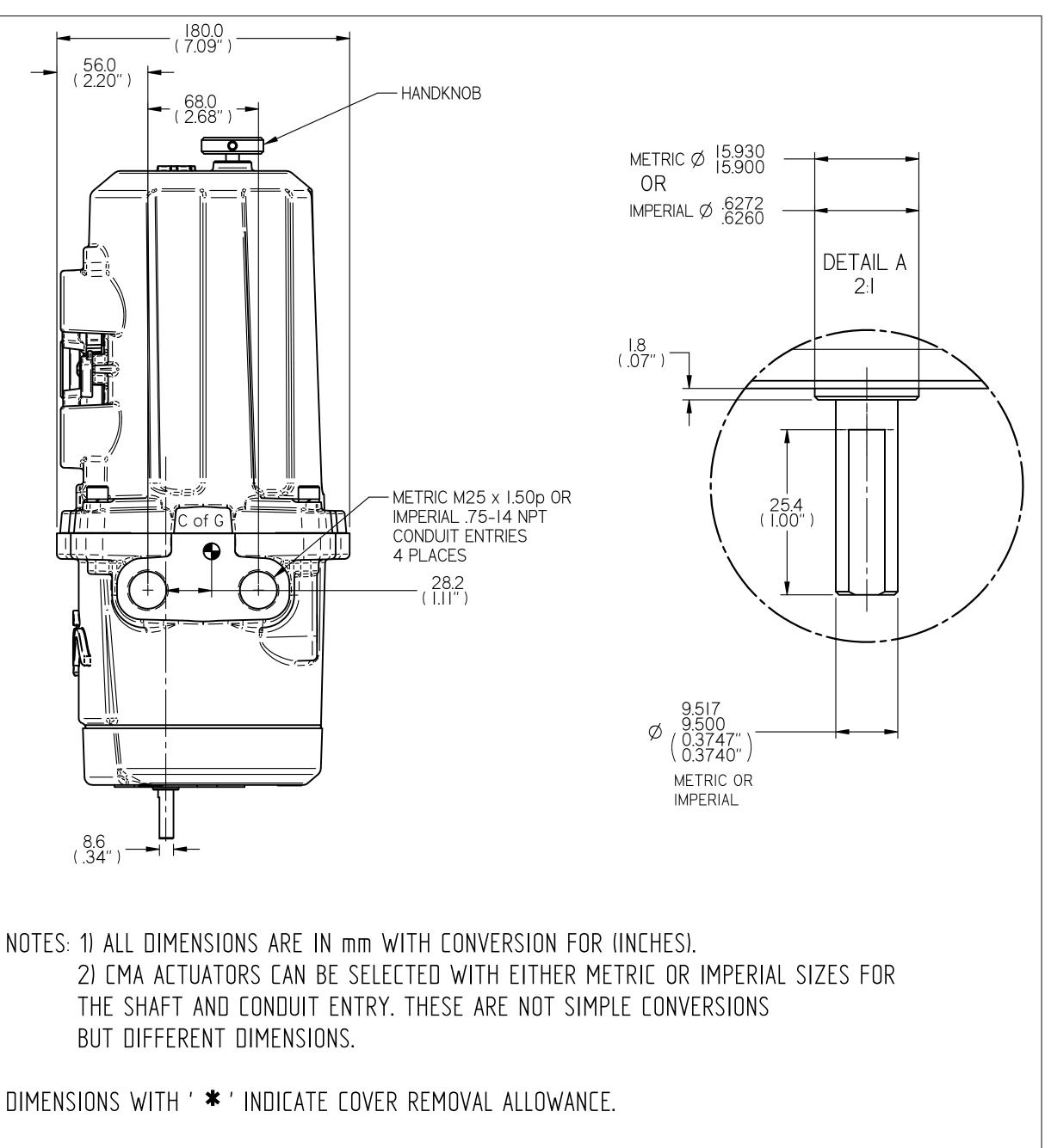
THE INTERFACE PROVIDED FOR MOUNTING THE ACTUATOR ON TO THE VALVE SHOULD CONFORM TO GOOD ENGINEERING PRACTICES, ENSURING ADEQUATE TOLERANCES, THREAD ENGAGEMENT, SCREW TORQUES, SIZES, MATERIALS & FORM TOLERANCES. NOTE 200 IN LBS MAY
