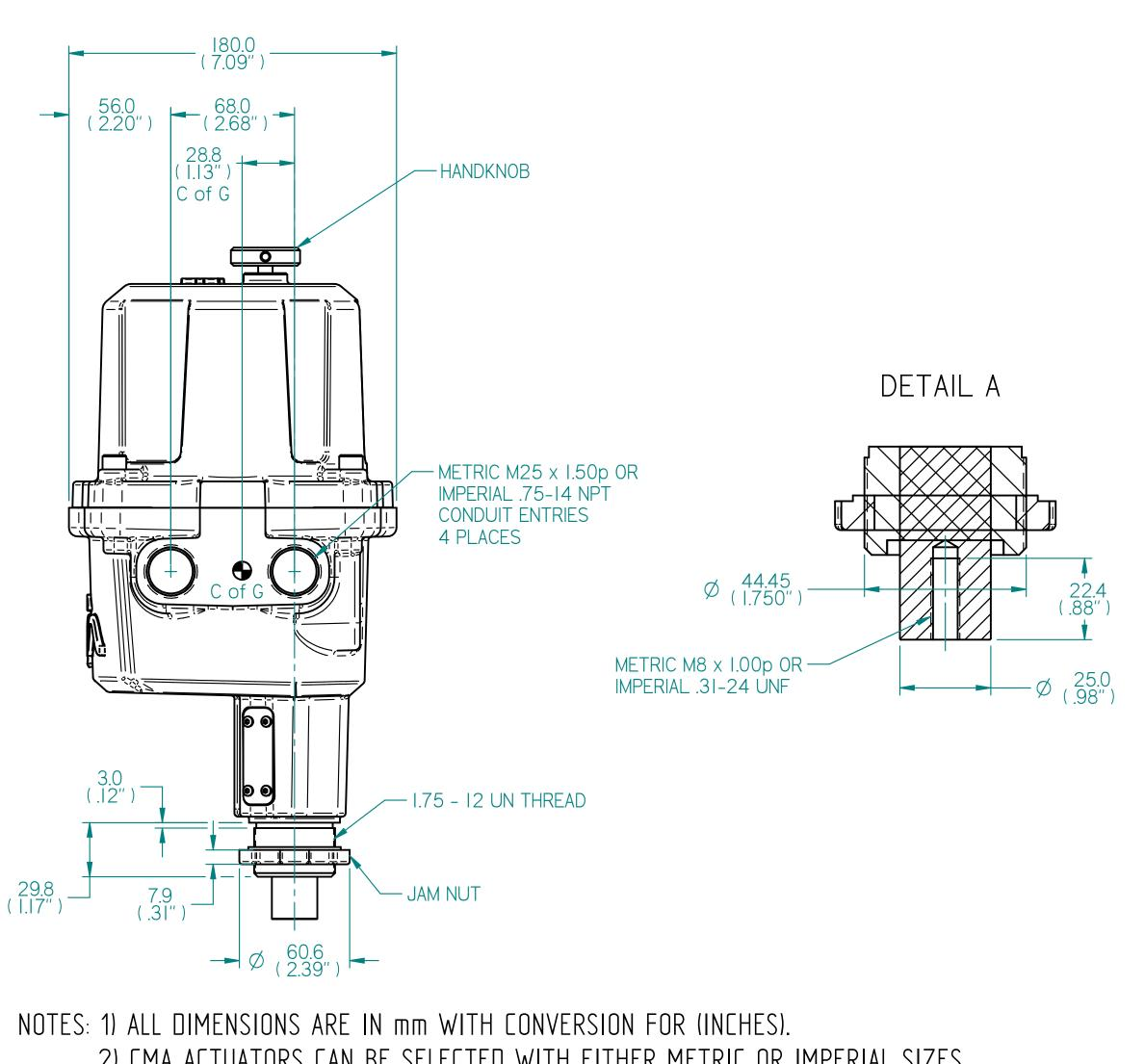
2) CMA ACTUATORS CAN BE SELECTED WITH EITHER METRIC OR IMPERIAL SIZES FOR MOUNTING, SHAFT AND CONDUIT ENTRY. THESE ARE NOT SIMPLE CONVERSIONS BUT DIFFERENT DIMENSIONS.
